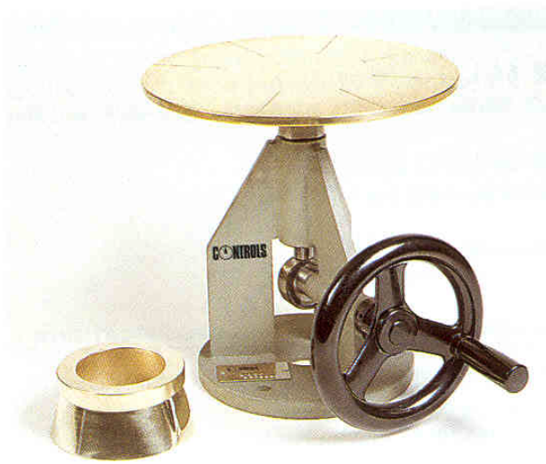
a) Flow Test Equipment
